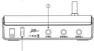
power cable buckle: the power cable can be fixed to avoid accidentally falling off.
