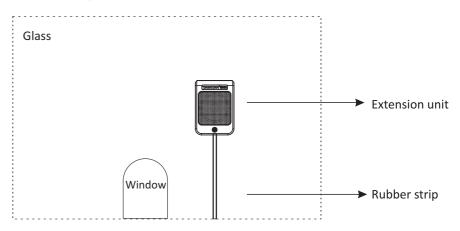
Keep the wall and glass clean to prevent the rubber strip from falling off due to the dust on the wall or the glass, keep the connecting cable connector of the extension unit downward and put the cable into the slot of the rubber strip, paste the rubber strip on a proper position outside the window, drill a screw hole on the wall and fix the extension unit via screw, or fix the extension unit on the glass via the supplied adhesive EVA foam.
